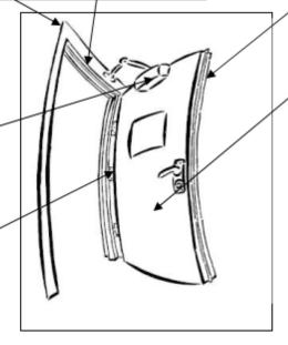
BS 476 fire door hung with regular 3mm gap between it and the frame.
